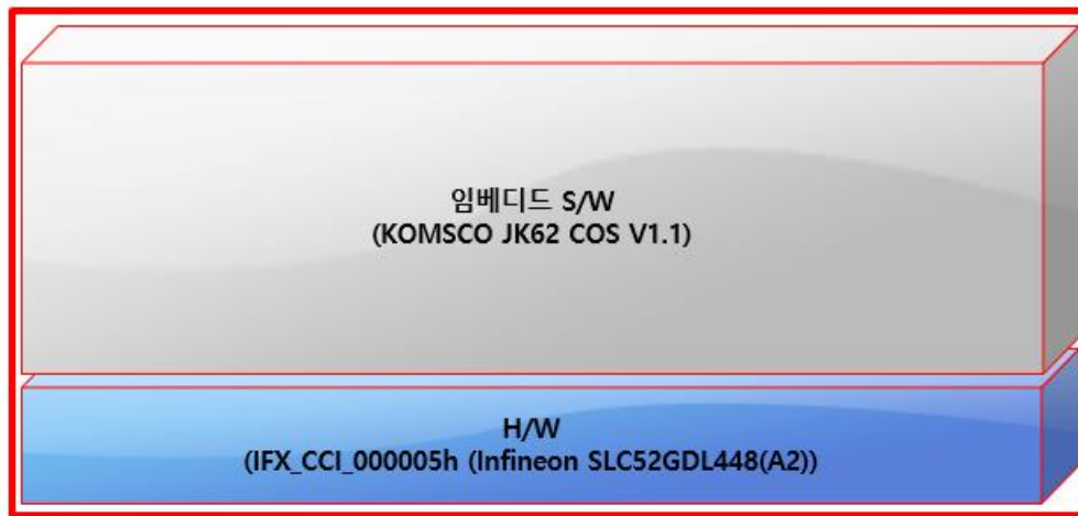
[Figure 2] Architecture of the TOE
